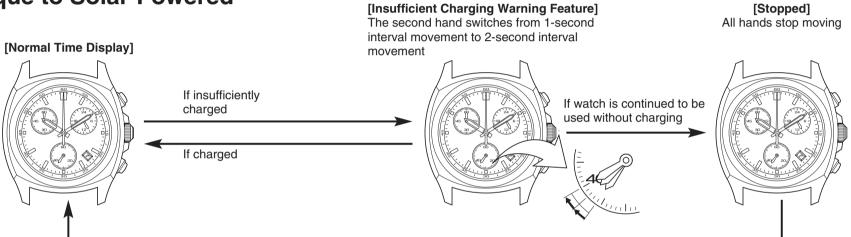
The watch hands resume 2-second interval movement when the watch is charged by exposing to light. However, the time is incorrect as a result of the watch having stopped due to being insufficiently charged. Sufficiently charge the watch until it resumes 1-second interval movement and reset the time before use.
